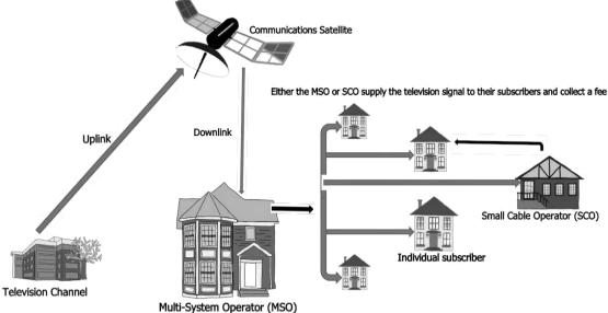
Fig 1. Diagram of a simple cable network system
