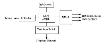
Fig 2 Equipment located at the head end
