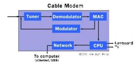
Fig 4. The Internal structure of a cable MODEM
